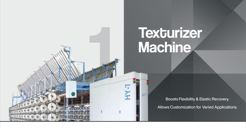
A **Texturizer Machine** in the textile industry is used to modify the physical properties of fibers and yarns, enhancing their appearance, strength, and usability.
