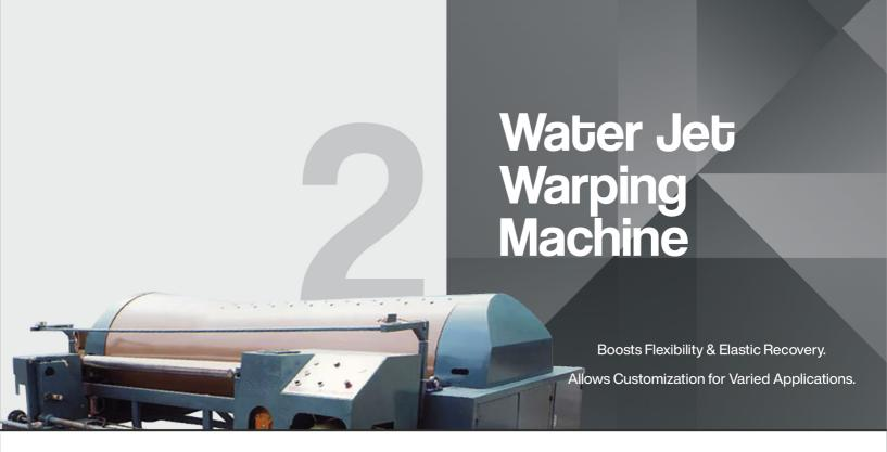
A **Water Jet Warping Machine** is used in the textile industry for warping yarns efficiently before weaving. It utilizes a high-pressure water jet system to achieve uniform tension and arrangement of yarns.
